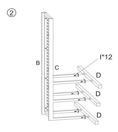
2-Fasten beams (D) to the frames (B & C) with screws (I).
